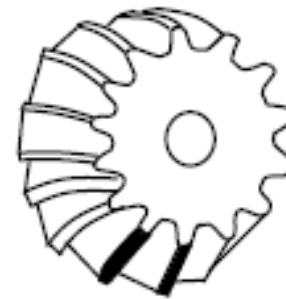
(b) Zerol Bevel Gear
